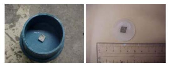
Fig. 2.2.5 Final Test Piece Set in Hard Epoxy.
